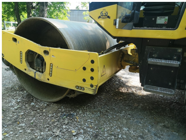
Fig. 3. Echipament compactor cu rulou vibrator
