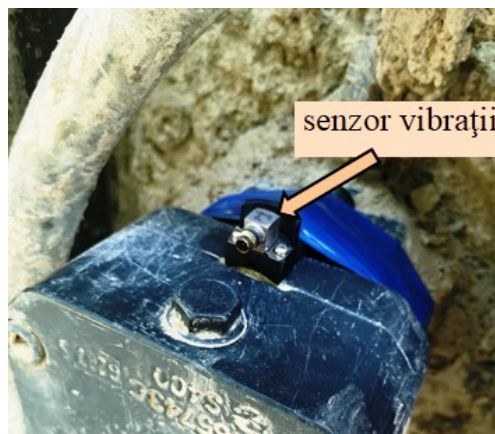
Fig. 3. Echipament compactor cu rulou vibrator
