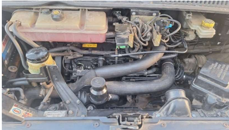
Fig. 2 Motorul Diesel 2.0 l common rail testat
