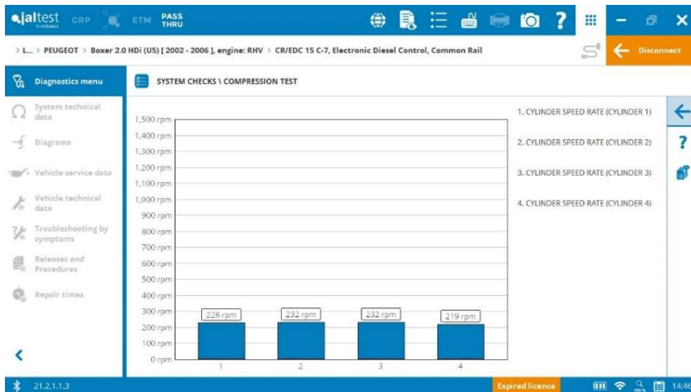
Fig.4 Test electronic de compresie
